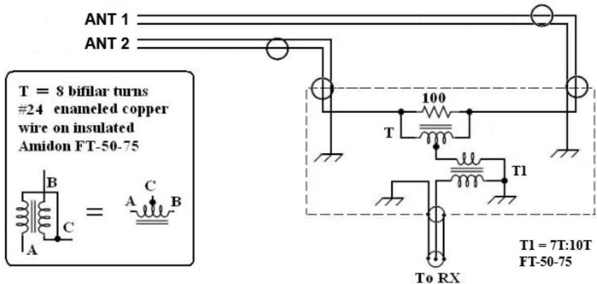
This picture shows connection of the wires in the combiner transformer **T**
