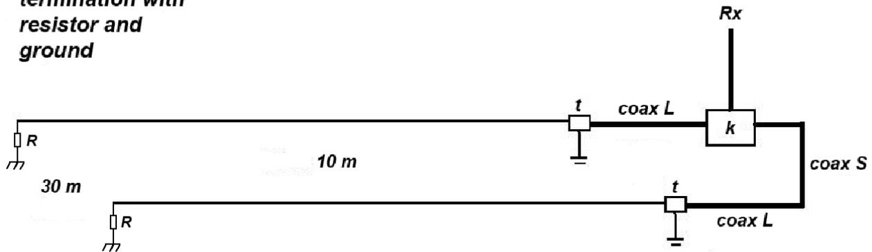
The figure shows a staggered beverage array where the desired signals are coming from the left. The offset is 30 m and the distance between the beverages is 10 m.
