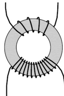
The core type used determines the number of turns. The figures and turns shown are for FT50-75 cores.
